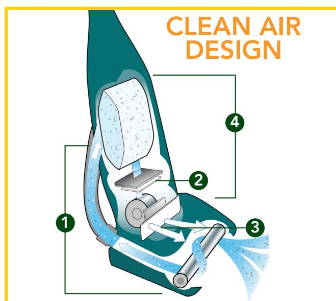
1. Dirt is pulled in and drawn through the vacuum bag.
